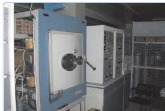
Arc discharge UVNIPA-1-001 sputtering system
